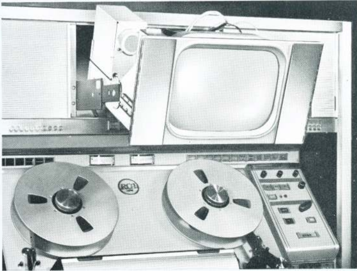
Slide and tilt mounted monitoring — accessibility plus.
